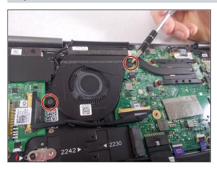
Remove the two screws holding the cover for the fan.
