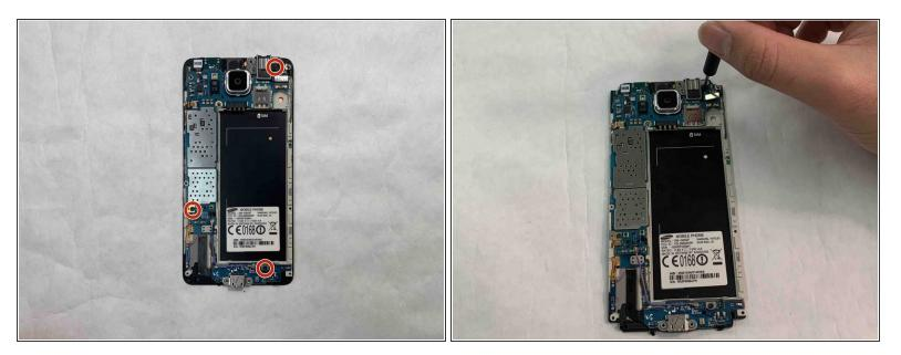
Using the Phillips #00 screwdriver, remove and set aside the three 3.0 mm screws that secure the motherboard to main phone body.
