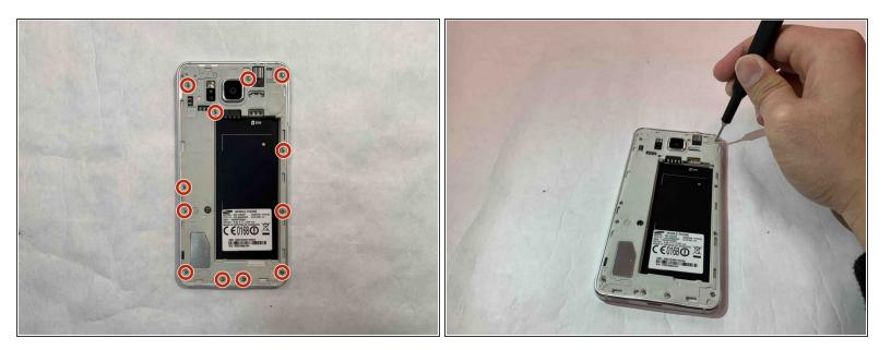
Using the Phillips #00 screwdriver, remove and set aside the twelve 3.0 mm screws that secure the back case to the main phone body.
