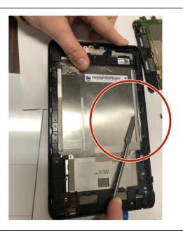
Using a guitar pick or a metal spudger, remove the old screen from the device from the back of the tablet.
