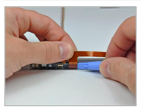
Use a plastic opening tool to pry the camera ribbon cable away from the camera board.
