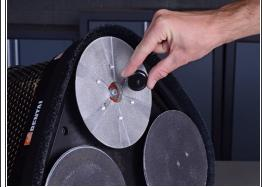
Use a flathead screwdriver to pry off and remove the rubber plug in the center of the sanding disc.
