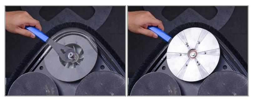
Slide a thin 22 mm wrench underneath the sanding disc and clasp it onto the flat part of the motor driveshaft to keep the driveshaft from turning.
