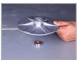
Place a 15/16" socket inside the center of the sanding disc and use a mallet to tap the bearing out of the disc.
