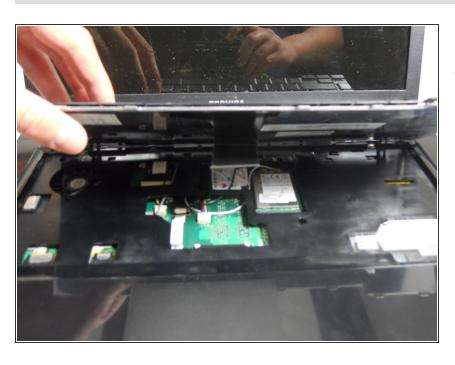
With the black ribbon cable now disconnected, remove the keyboard from its housing. Congratulations, you have removed the laptops original keyboard and can now replace it with a new one.
