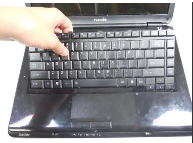
Starting at the top, gently raise the keyboard enough to remove it from the socket.
