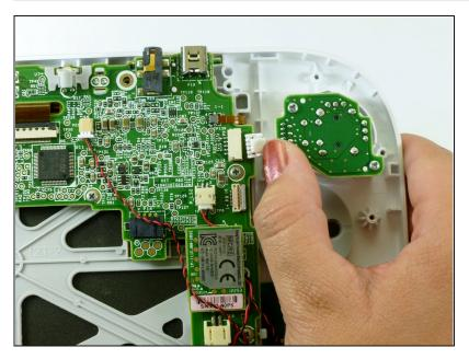
Use your thumb and push the connector towards the rightmost edge to disconnect the analog stick cable connector.
