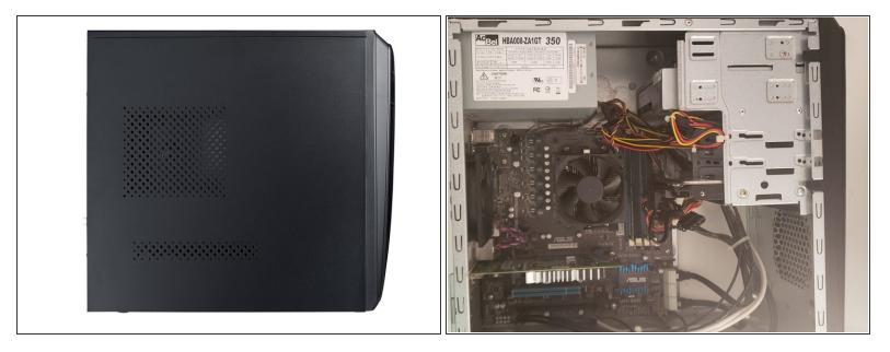
• Remove the sidepanel by unscrewing the two screws fastening the panel on the rear. Once unscrewed, slide the panel towards the rear until it releases then lift away.
