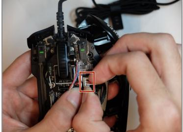
Remove the top housing LED 3-Pin connector that is near the main board.
