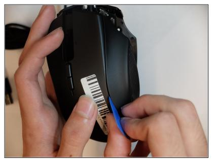
Remove the side housing using the opening pick.
