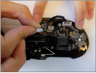
Remove the scroll wheel optical encoder 3-pin connector from the main board by wiggling the connector upwards.
