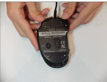
• Remove the mouse's feet using the opening pick.
