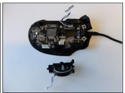
Using the opening tool, pry the black bracket holding the scroll wheel in place backwards until the scroll wheel housing pops out.
