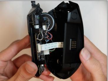
Separate the top mouse housing from the bottom mouse housing using the opening pick.
