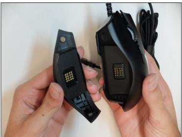
Remove the interchangeable side plate.
