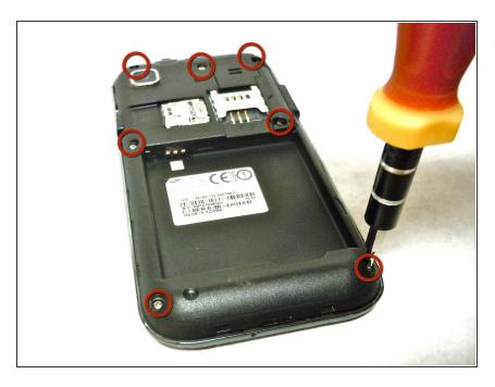
Remove the seven 4.5 mm Phillips #00 screws along the perimeter of the phone.
