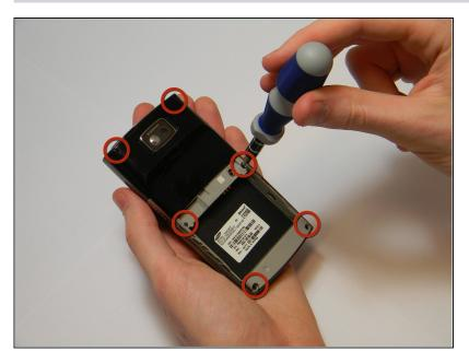
Remove the six 4.0 mm screws using the Phillips 00 screwdriver.
