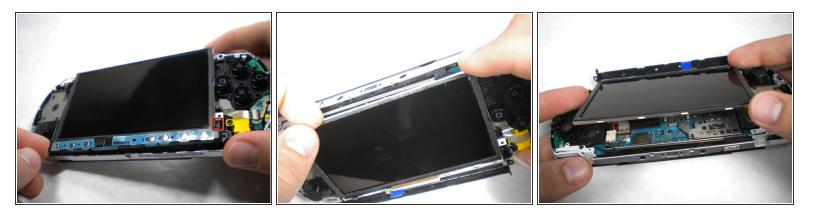
• Push the homebar to the right to release the tab on the right side of the LCD screen.
