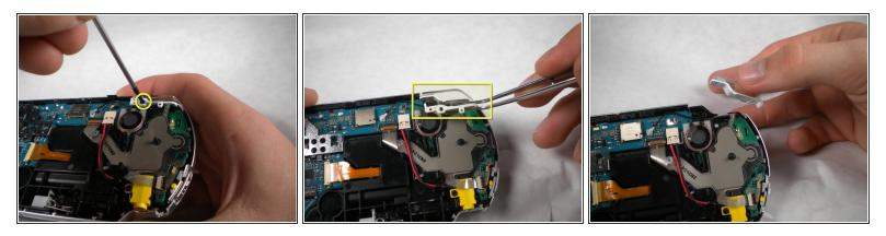
• Unscrew the 'R' trigger and remove both pieces. (Refer to step nine by applying the procedures to this, the right, side)
