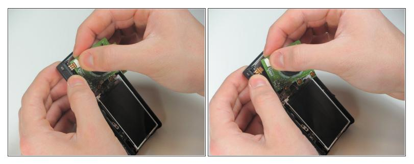
Using your hand, or a pair of tweezers, remove the ZIF connector by gently pulling it out of the dock on the circuit board.
