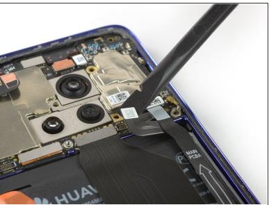
Use a spudger to pry up and disconnect the battery connector.
