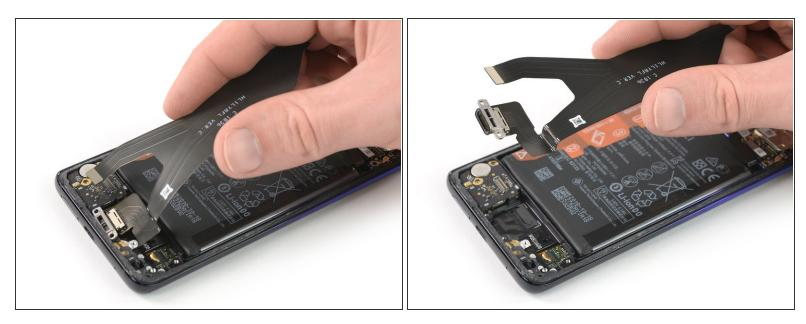
Remove the main flex cable including the charging port by lifting it upwards and then pulling it in the direction of the motherboard.
