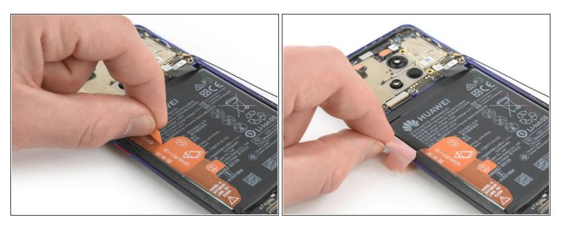
Peel the orange adhesive strip labeled with a 1 off the battery. The orange adhesive tape will rip along a small perforated line.
