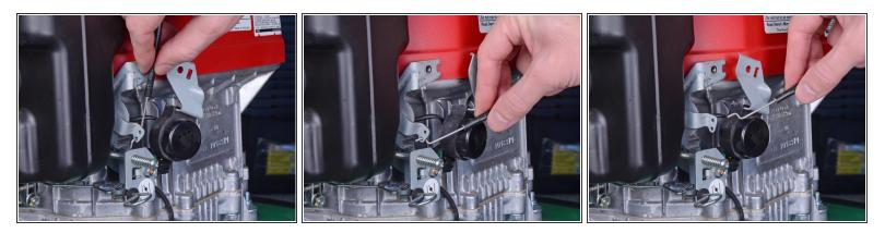
• Rotate the lower end of the throttle cable to detach it from the throttle.
