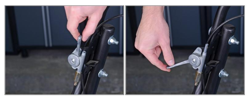
• Advance the throttle control to expose the gear rack containing the upper end of the throttle cable.
