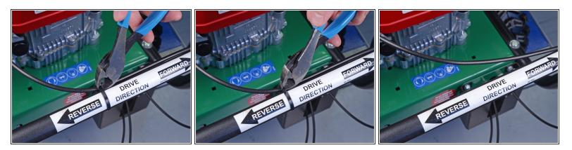
• Cut and remove any zip ties securing the throttle cable.
