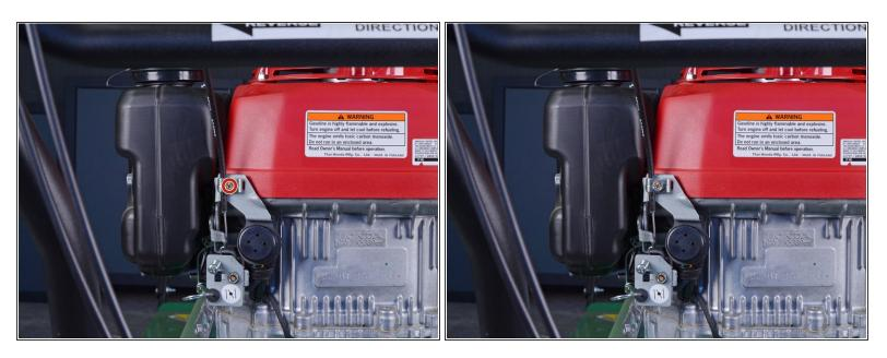
Use a Phillips #2 driver to remove the screw securing the lower end of the throttle cable.
