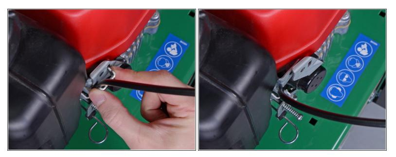
• Remove the bracket securing the lower end of the throttle cable.
