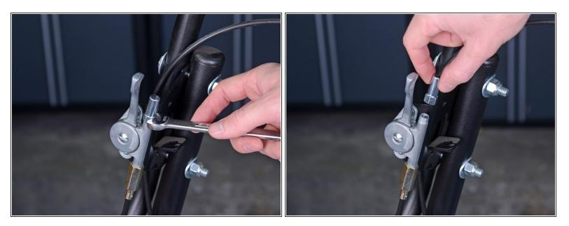
■ Use a 7/16" wrench or deep socket to remove the cap from the throttle control.
