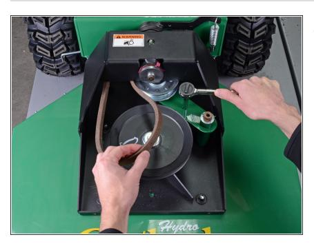
Slip the belt off the deck pulley.
