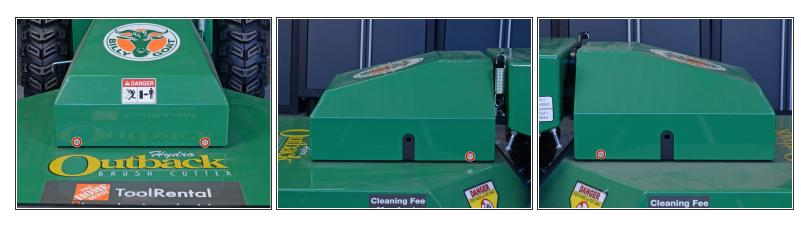
Use a 3/8" socket or wrench to remove the four 21 mm bolts securing the cover to the deck—two at the front, and one on each side.
