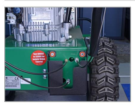
Use a 1/2" socket or wrench to remove the two 26 mm bolts securing the rear guard to the back end of the brush cutter.
