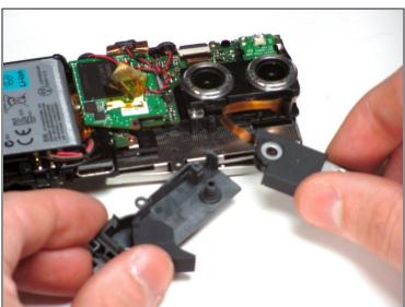
• Carefully lift the USB drive off of the peg that it is attached to.
