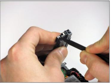
• Using a spudger, remove the clips of the metal casing from each end of the USB drive.
