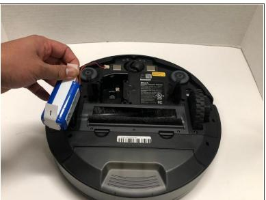
• Disconnect the battery from the device by pulling it out of the circuit.
