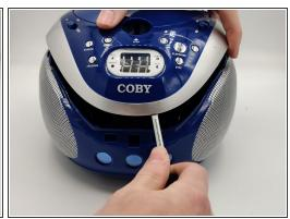
Pry open the top portion of the case using a spudger.
