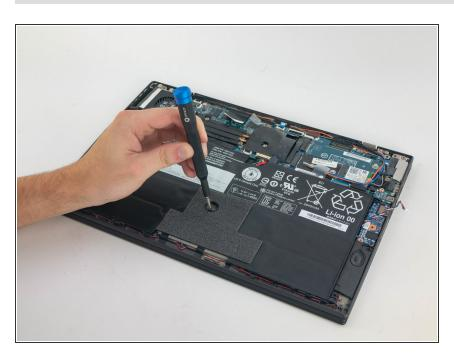
Using a Phillips #0 screwdriver, unscrew the five 4.3mm screws attaching the battery to the computer.
