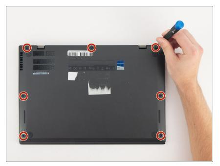
Using a Phillips #0 screwdriver, remove the seven 7mm screws holding the back cover onto your computer.
