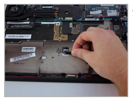
Remove the black ribbon cable connected to the touchpad.
