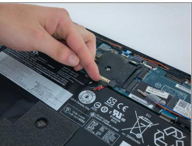
Using your fingers, disconnect the battery from the motherboard.
