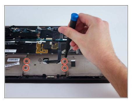
Use a Phillips #1 screwdriver to remove the four 1.9 mm screws holding in the touchpad.
