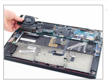
Remove the fan by lifting it directly up.
