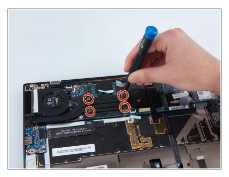
Use a Phillips #1 screwdriver to undo the four 5 mm screws attached to the heat sink.
