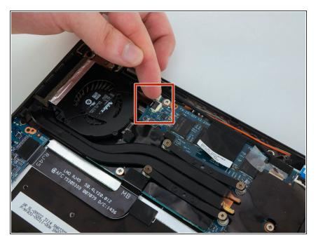
Undo the black clasp that holds the ribbon cable, attached to the fan, in place and disconnect the ribbon cable.
