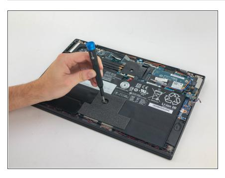
Using a Phillips #0 screwdriver, unscrew the five 4.3mm screws attaching the battery to the computer.
