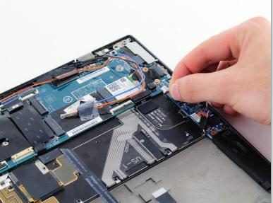
Disconnect the wire connecting the motherboard to the speaker.
