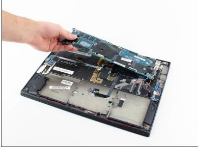
• Carefully remove the motherboard by lifting it and pulling towards the left.
