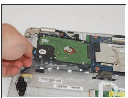
Pull up on the ribbon beneath the hard drive to lift the hard drive upwards.
