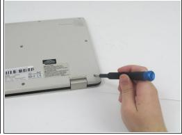
Use a Phillips #1 screwdriver (PH1 bit) to remove the ten 5mm screws that secure the bottom cover.
