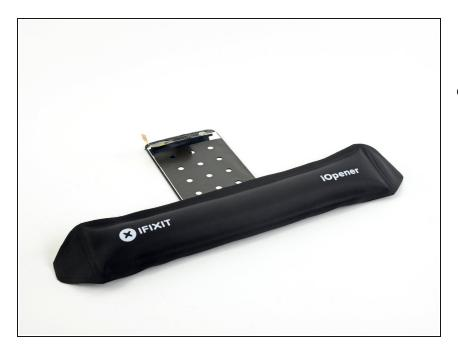
Apply a heated iOpener to the fingerprint sensor for one minute to soften the adhesive gasket.
