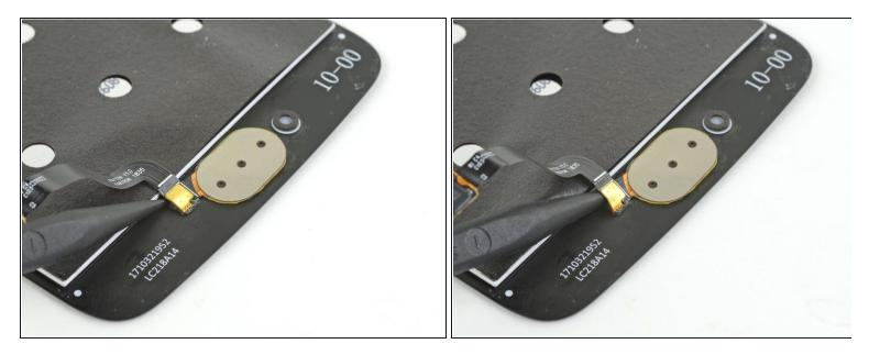
• Slide the point of a spudger under the fingerprint sensor cable and gently pry to loosen the cable from the screen.
