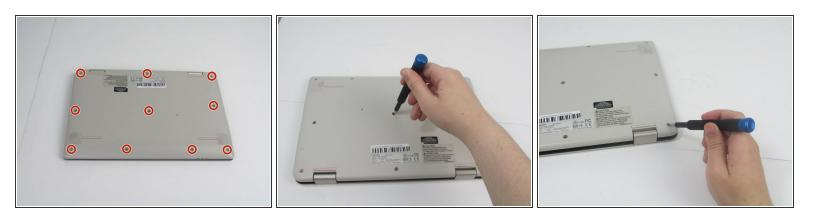
Use a Phillips #1 screwdriver (PH1 bit) to remove the ten 5mm screws that secure the bottom cover.
