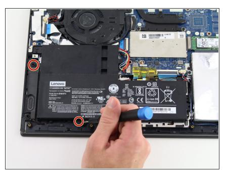
Remove the two 3.6 mm Phillips #00 battery screws located in the lower left corner of the device.
