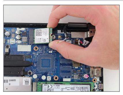
• Remove the wireless network adapter.
