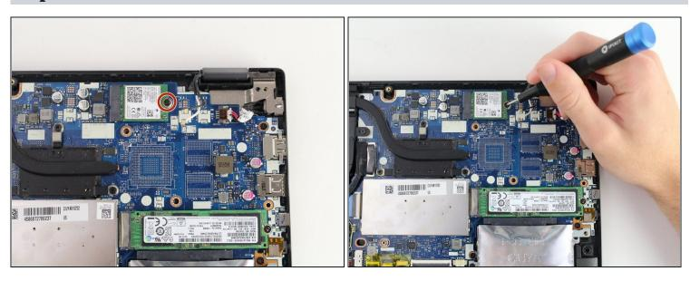
• Using the Phillips #00 screwdriver, remove one 3.6 mm screw.
