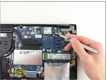
• Use the reverse <u>tweezers</u> to carefully unplug the two wired connections.
