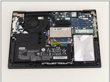
Use the plastic opening tool to lift up and remove the casing.
