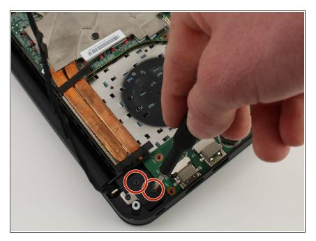
Remove the two 5mm Phillips #00 screws.
