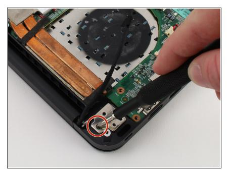
• Remove one 3mm Phillips #00 screw from the metal plate.
