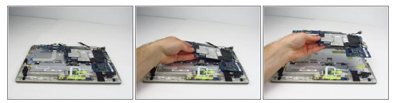
• To remove the motherboard from the casing, gently lift the left side and pull it out of the casing.
