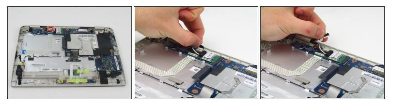
• Gently remove the insert next to the wi-fi card on the motherboard. Use your fingernails to gently pull on the tabbed insert, and place it out of the way.
