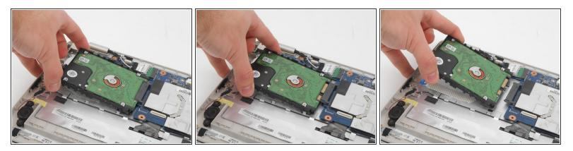
Gently pull the hard drive towards the edge of the laptop to disconnect the hard drive from the laptop circuitry.
