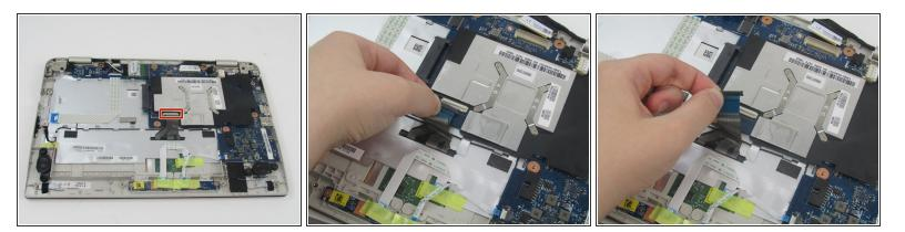
• Carefully remove the blue ribbon cable attached to the silver plate on the motherboard using your fingernails to gently pull on the tabbed insert, and place it out of the way.
