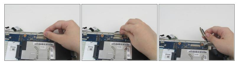
• Grab the paper tab on the cable near the silver part of the motherboard. Gently pull it away from the slot, and place it out of the way.
