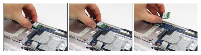
• Pull on the sides of the WiFi card to remove it from its slot on the motherboard. Lift the card out and up away from the motherboard, as it will try to bend back into the casing.
