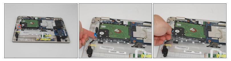
• Pull up on the ribbon beneath the hard drive to lift the hard drive upwards.
