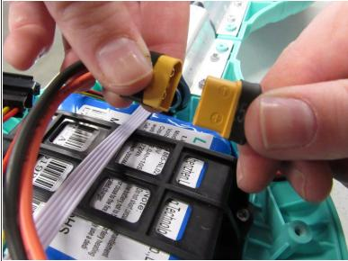
Disconnect the battery to prevent any electrical currents from coming through the wires.
