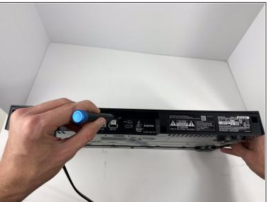
Using the Phillips #2 Screwdriver, remove the six 9mm screws from the back of the device.
