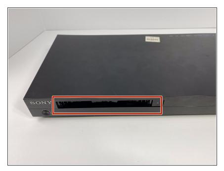
Remove the disk tray cover from the device.
