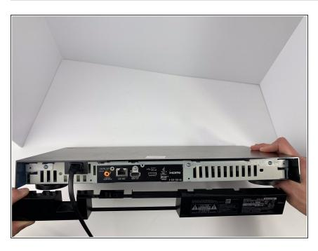
Pull off the back panel and remove it from the device.
