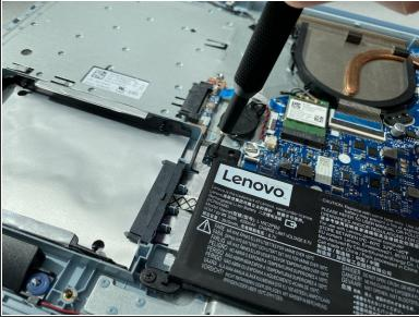
Using a Phillips #0 screwdriver to unscrew the four 5.5 mm screws securing the battery.
