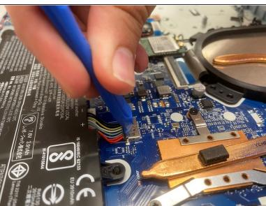
Disconnect the battery cable from its motherboard socket by gently pulling it towards the battery.
