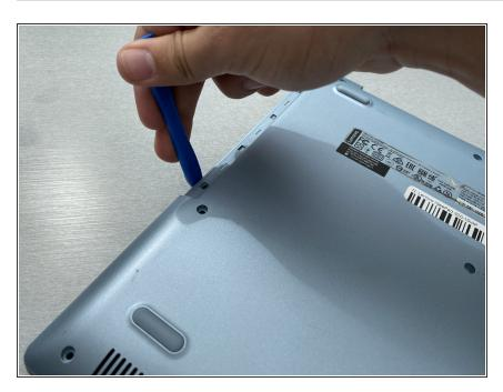
Lift up the cover using the opening tool on different spots along the side of the laptop.
