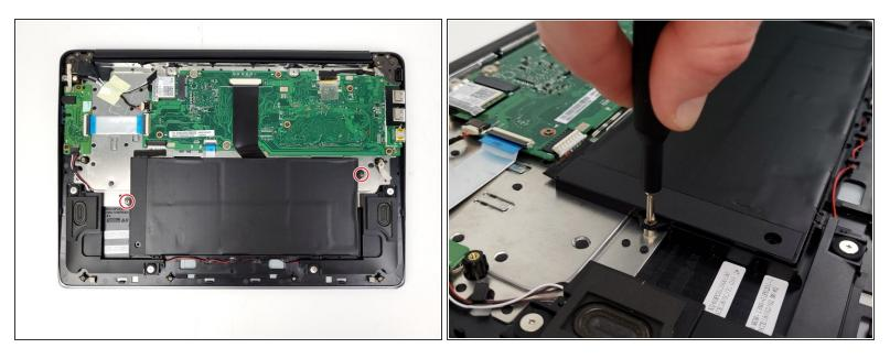
Use a Phillips #0 screwdriver to unscrew the two 5.5mm screws from the battery housing.
