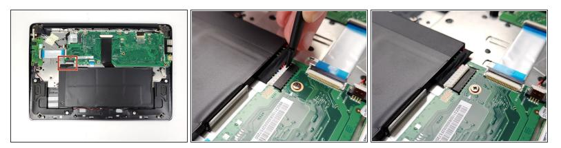
Use a spudger to disconnect the battery's connector from the motherboard. The connector should slide out toward the battery.
