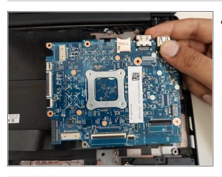
Gently remove the motherboard by hand from the base of the device.
