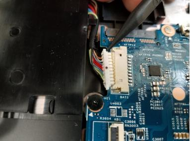
Remove the battery connector by pushing both ends away from the motherboard one at a time using the pointed end of a spudger.
