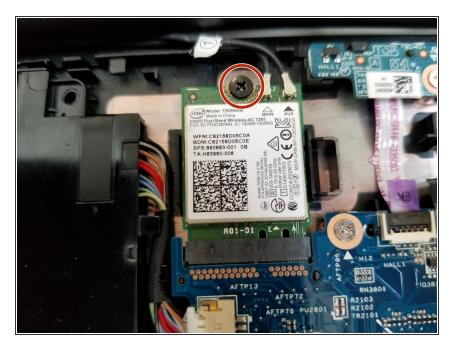
Remove the 4mm screw from the Wi-Fi card using a Phillips #00 screwdriver.
