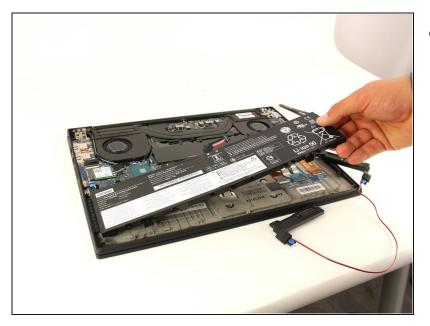
Lift the battery out of the frame and remove it from the device.
