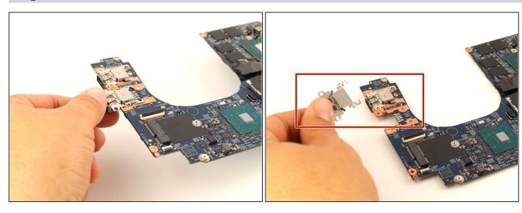
• Gently push the docking station towards the center of the motherboard, lift up to release a lock, then pull it out to remove it from the device.
