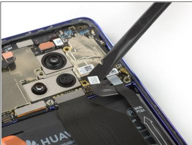
Use a spudger to pry up and disconnect the battery connector.
