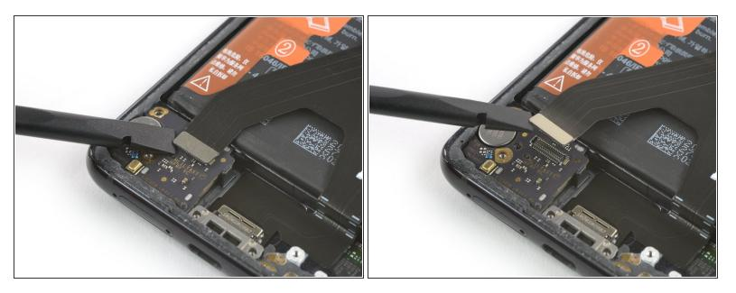
• Use a spudger to pry up and disconnect the main flex cable from the left daughterboard.
