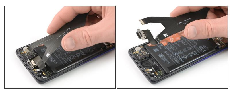
Remove the main flex cable including the charging port by lifting it upwards and then pulling it in the direction of the motherboard. If possible, turn on your device and test your repair before installing new adhesive and resealing.
