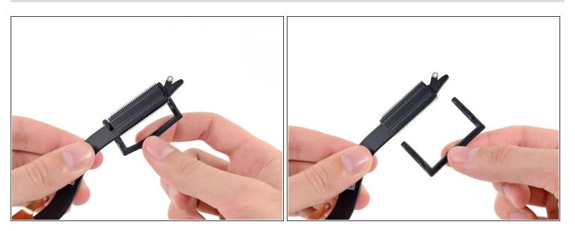
Carefully remove the right fan duct from the edge of the heat sink.
