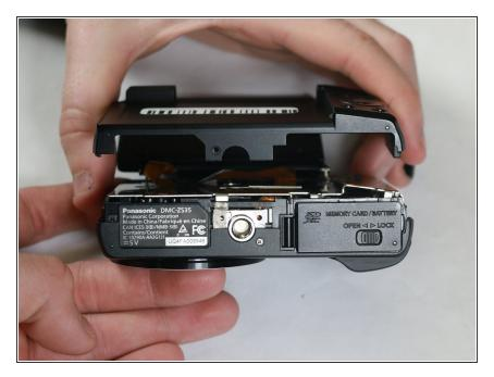
Gently pry apart the back casing from the body of the camera. It's recommended to apply as minimal force as is necessary to prevent unintended damage to the camera or the casing.
