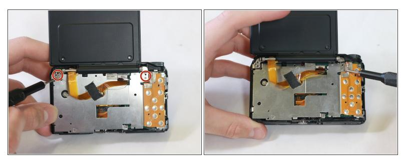
Unscrew the four 3mm screws holding the LCD screen hinge in place using a Phillips #000 screwdriver.
