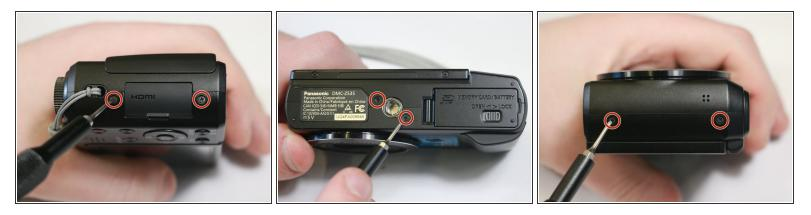
Remove the six 4mm screws located on the side and bottom of the camera casing using a Phillips #000 screwdriver.
