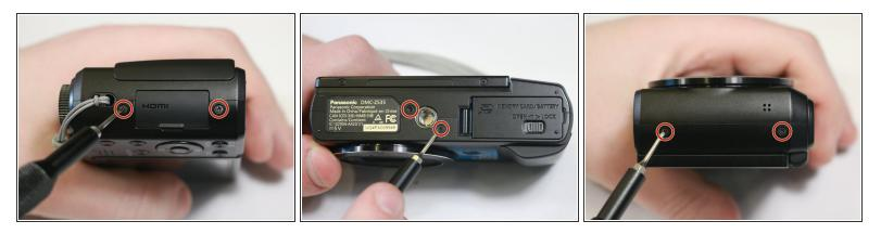
Remove the six 4mm screws located on the side and bottom of the camera casing using a Phillips #000 screwdriver.
