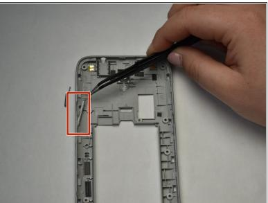
Use the curved tweezers to pull upwards and out on the the thin plastic attached on both sides of the power button and volume buttons. This process should allow the buttons to pop right out.
