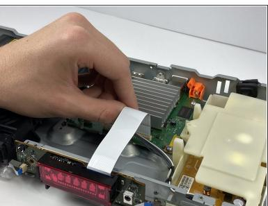
Unplug the large ribbon cable connecting the front panel board to the motherboard.
