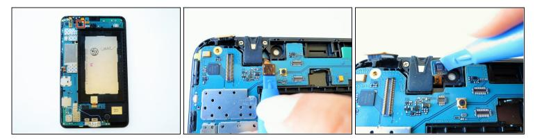
• Slightly apply pressure and move the blue plastic opening tool downwards to pop the gold square connector from its socket on the mother board.
