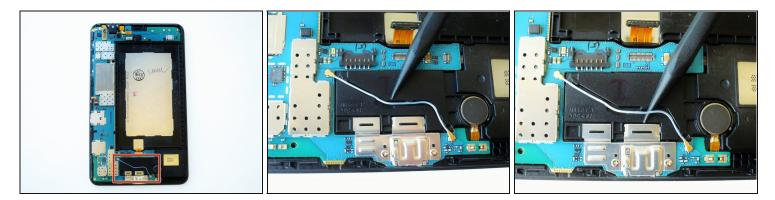
• Using the spudger gently wedge the blue wire out of its compartment.
