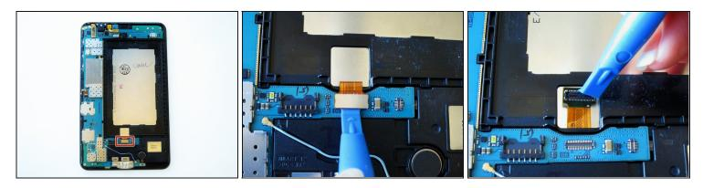
• Slightly apply pressure and move the blue plastic opening tool downwards to pop the metallic rectangular connector from its socket on the mother board.
