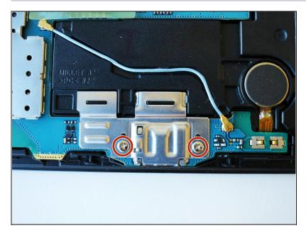
Remove two 2 mm #000 Phillips screws securing the metallic charger port cover to both the logic board and the front panel.
