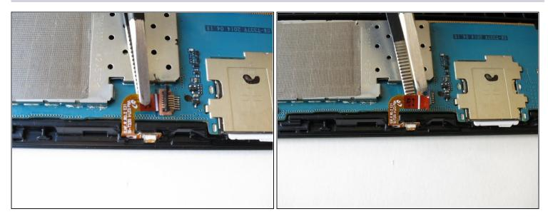
• Squeeze the golden cable with the tweezers and gently pull the cable to the left to free the end of the golden cable.
