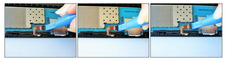
• Carefully insert the flat end of the blue plastic opening tool under the black plastic fastener and lift.
