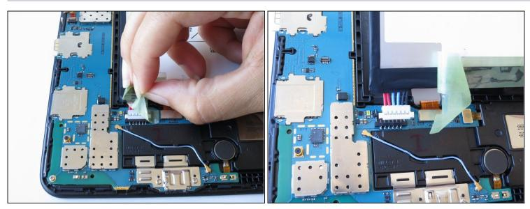
• Starting at the bottom left side of the battery, gently remove the green tape.
