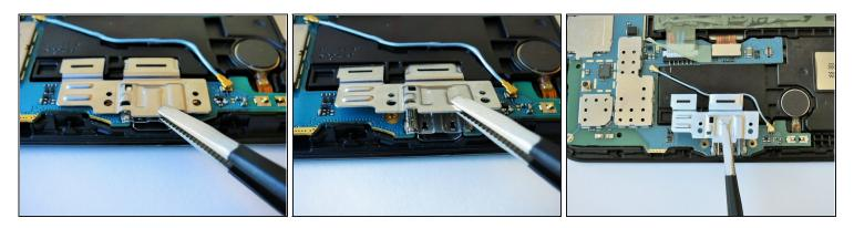
• Squeeze the metal charger port cover piece with the <u>tweezers</u> to gently lift it from it's place.
