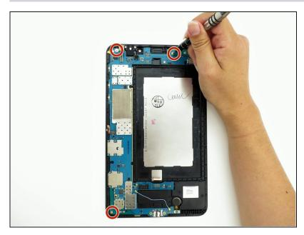
Remove three 2 mm #000 Phillips screws securing the mother board to the front panel.
