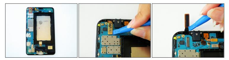
• Slightly apply pressure and move the blue plastic opening tool downwards to pop the gold rectangular connector from its socket on the mother board.
