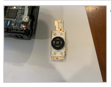
Gently remove buttons by hand, once all of the screws holding the buttons in are removed.
