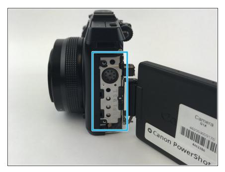
Remove the side panel covering the speaker by gently pulling it away from the camera. You can also use spudgers to create a lever to help remove the panel.
