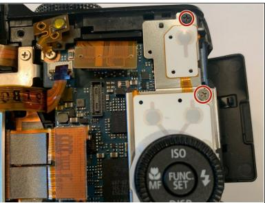
Remove the two screws above the buttons followed by the screw on the bottom, using a Phillips #00 screwdriver.
