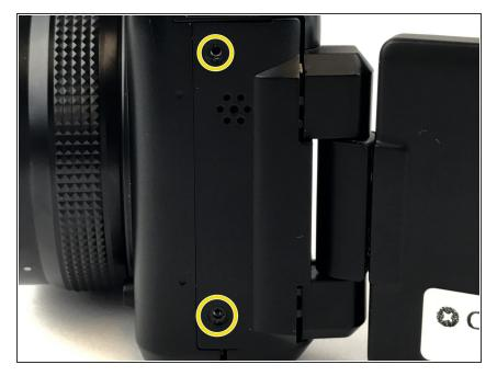
Now flip to the opposite side of the USB panel screw and unscrew the two screws holding the small speaker cover portion of the camera. Use a Phillips Head 00 screwdriver for both of these screws.
