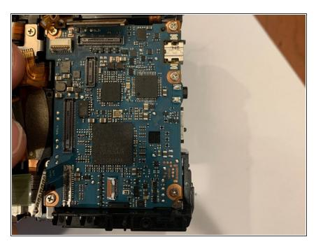
Remove the ribbon wire that is on top of the motherboard by gently pulling it out of its attachment.
