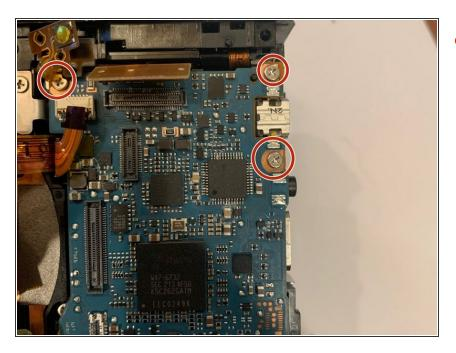
Remove the three screws on the top of the motherboard using a Phillips #00 screwdriver.
