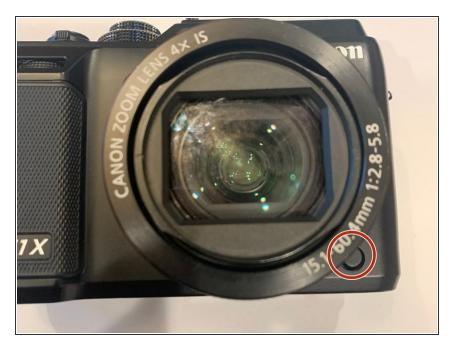
Remove the Canon Zoom Lens by pressing this button down while pulling the lens up.
