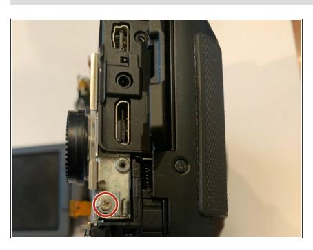
Remove the screw on the side of the buttons using a Phillips #00 screwdriver.
