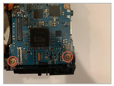
Remove the bottom two screws on the motherboard using a Phillips #00 screwdriver.
