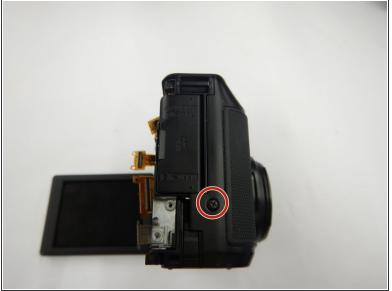
Remove the two screws on the front casing using a Phillips #00 screwdriver.
