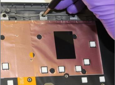
Using the Phillips #1 screwdriver, remove 23 (twenty three) 4.5mm screws.
