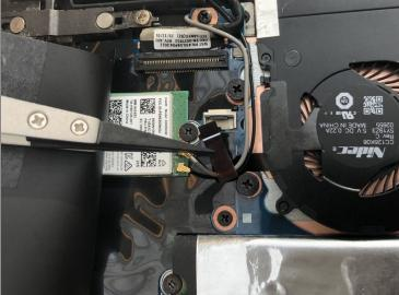
• Using <u>tweezers</u>, pull the plastic strip out.
