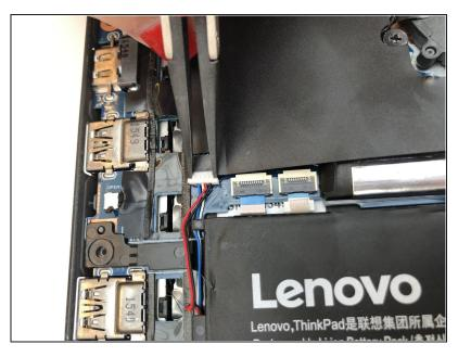
Using a pair of <u>tweezers</u>, push the sides of the white speaker wire toward the battery (where it says Lenovo) to unplug it.
