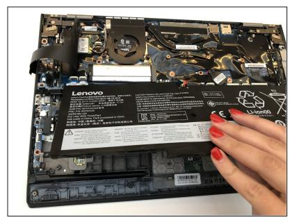
• Lift and remove the battery away from the computer.
