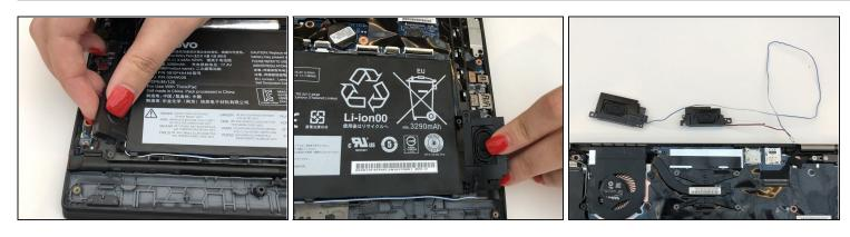
• Remove the speakers from either side of the battery. The connecting wire will unthread from the sides of the battery.
