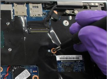
Using the Phillips #1 screwdriver, remove sixteen 4.5mm screws.
