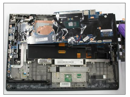
Lift and remove the motherboard away from the computer.
