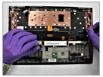
Using the iFixit opening tool, lift the metal frame away from the keyboard.
