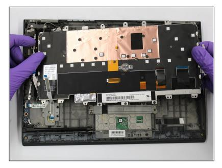
Lift and remove the keyboard away from the computer.
