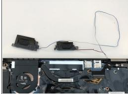
Remove the speakers from either side of the battery. The connecting wire will unthread from the sides of the battery.
