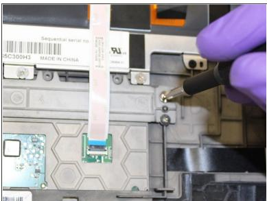
Using the Phillips #1 screwdriver, remove four 4.5 mm screws from the trackpad.
