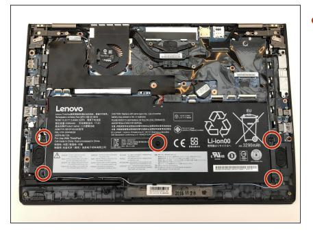
Remove the five 4.5mm Phillips #1 screws that secure the battery.
