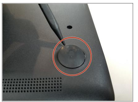
Remove four large rubber pads from the bottom of the device to reveal screws using the pointed end of a spudger.
