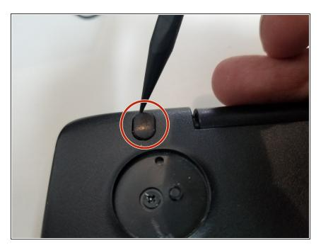
Remove two smaller rubber pads from the bottom of the device to reveal screws using the pointed end of a spudger.
