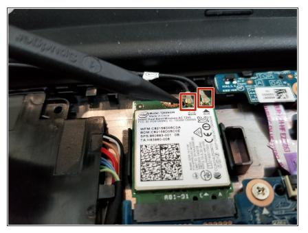
Remove the two wires from the top of the WLAN module by pulling them gently with a spudger or your hand and snapping the wires out of place.
