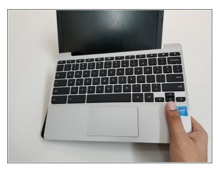
Gently remove the keyboard assembly by hand from the base of the device.
