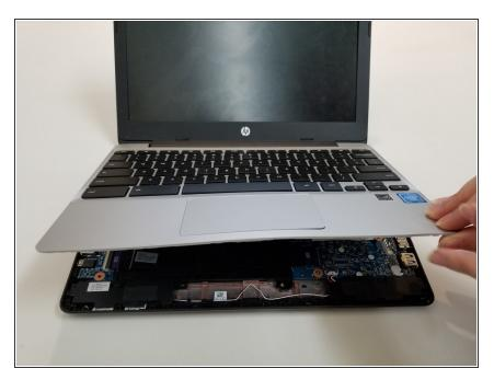
Gently lift the keyboard assembly slightly above the base of the device.
