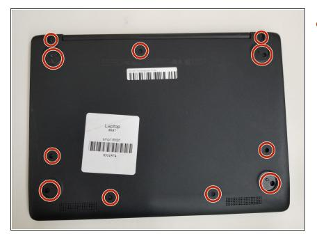
• Remove the 4mm eleven screws using a Phillips #00 screwdriver.
