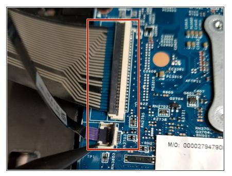
Disconnect the two ribbon cables connected to the motherboard by using the pointed end of a spudger to lift the plastic connector lids to allow the ribbon cables to be gently removed by hand.
