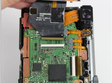
Use tweezers to pry up the black retaining flat and gently pull to free the LCD screen from the device.
