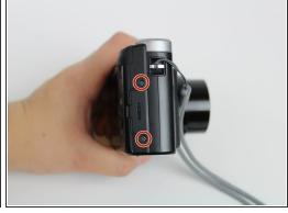
Using the Phillips #000 Screwdriver, unscrew six 3mm screws. There are two screws located on three sides excluding the top.
