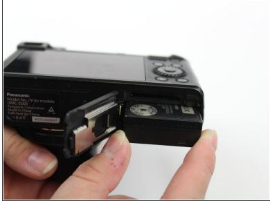
Push up the black tab on the right-hand-side to spring release the battery.
