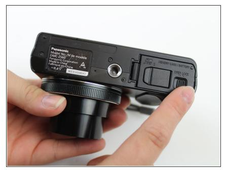
Use your finger to slide the black latch from the locked position to the open position on the memory card/battery door. This will open the door of the camera.
