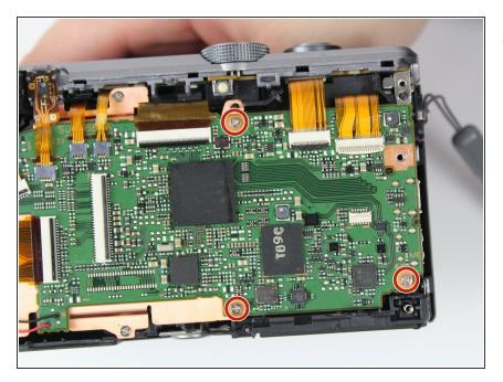
Remove these three 3 mm screws with a Phillips #000 screwdriver.
