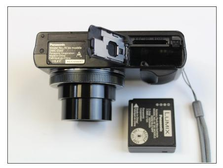
Remove the battery by sliding it out from the camera.
