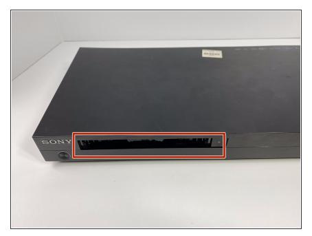
Remove the disk tray cover from the device.
