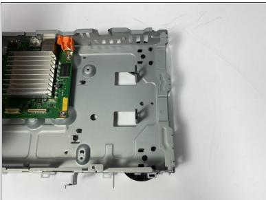
Remove the Power Supply Board.
