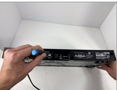
Using the Phillips #2 Screwdriver, remove the six 9mm screws from the back of the device.
