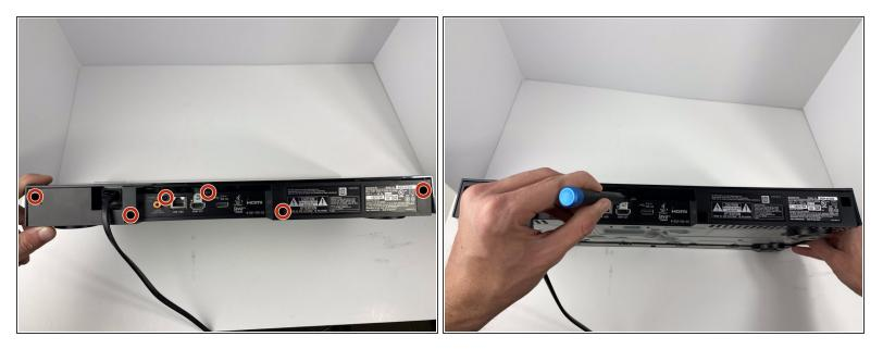
• Using the Phillips #2 Screwdriver, remove the six 9mm screws from the back of the device.
