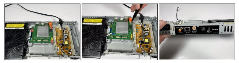
• Remove the three screws using the Phillips #2 Screwdriver.
