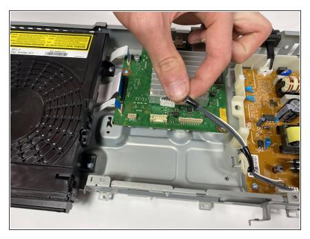
• Remove the cable connected to the power supply.
